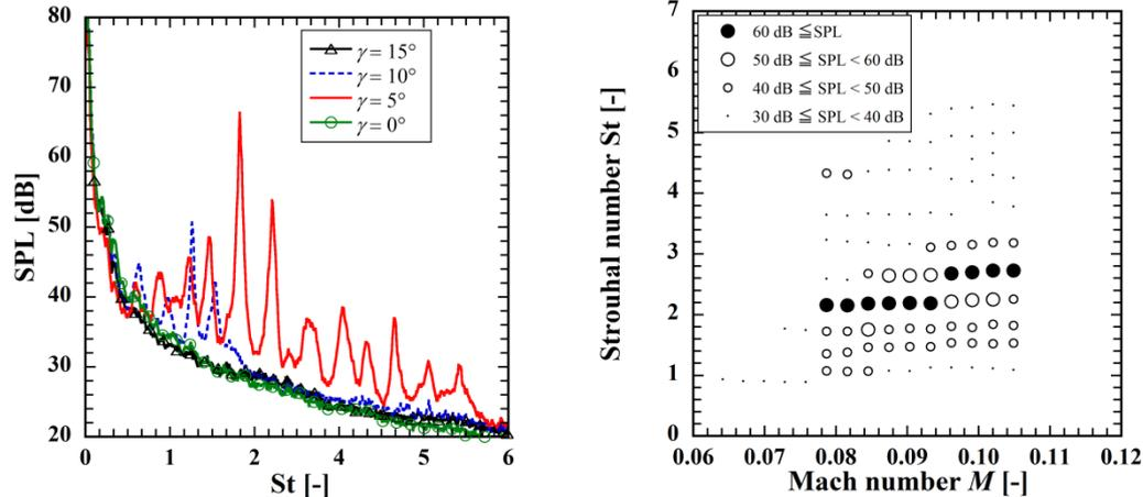
Figure 2 Measured sound pressure. (a) Sound pressure spectra ( $M = 0.087$ ,  $\Delta St = 0.01$ ). (b) Effects of Mach number on the fundamental frequency ( $\gamma = 5^\circ$ ).
