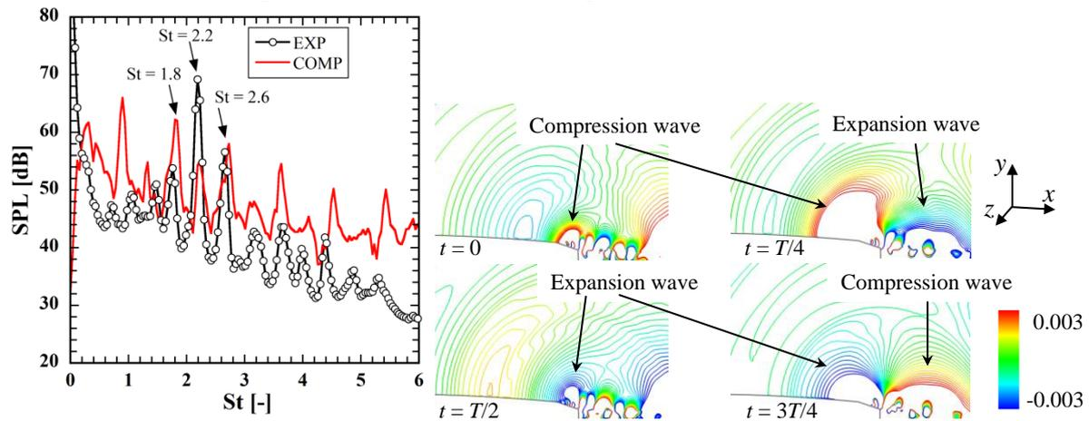
Figure 4 Acoustic fields ( $\gamma = 5^\circ$ ,  $M = 0.087$ ) (a) Sound pressure spectra ( $\Delta St = 0.04$ ). (b) Contours of predicted fluctuation pressure.
